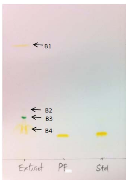
Fig.1: TLC for the extract and purified fucoxanthin (PF) compared with the standard commercial fucoxanthin (Std). B1-B4 represent for the bands of the pigments
